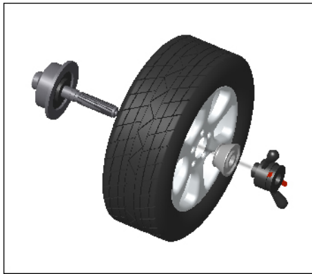
Front side installing
